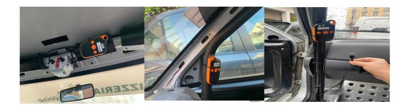
The GPS starts up when charging or with a long press of 5 seconds on the On/Off button located on the right side of the box (fig 1) the box vibrates and the LEDs flash: it is OK.
